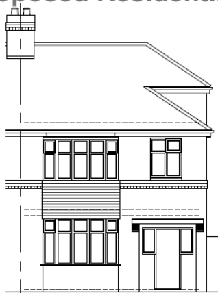
Existing Front Elevation
